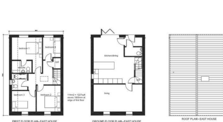
EAST UNIT - PROPOSED FLOOR & ROOF PLANS
